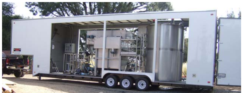
SAF™ System Pilot Trailer 200 gpm Treatment Capacity
