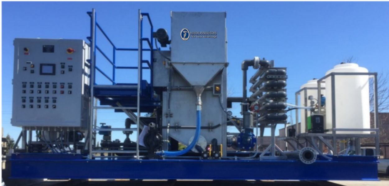
Figure 4. Suspended Air® Flotation Process – Entire Skid Mounted Water Treatment System; Inclusive of SAF Generator, Clear Floater, Serpentine Style Mixing Chamber, Chemical Staging, Polymer Mixer/Aging System, Floccmixer, Flowmeters, Solids Hopper, Pumps, PLC Cabinet and Maintenance Platform. (8' x 16' skid can accommodate up to 1,000 gpm)
